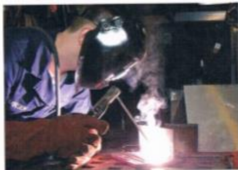
Welding beads with shielded metal arc welding
