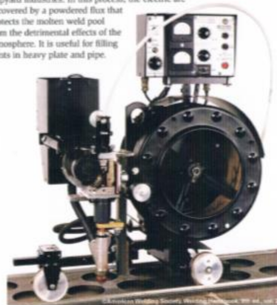
Self-propelled tractor used for submerged arc welding ships
