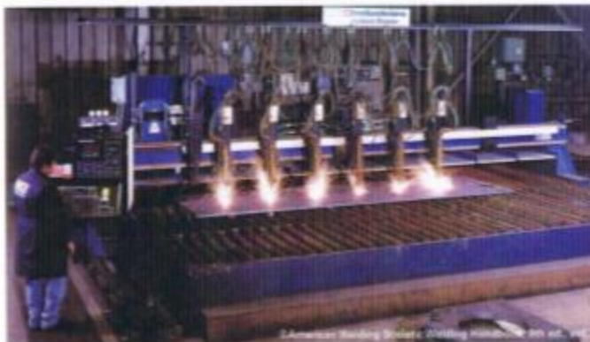
Cutting steel with an oxy-fuel torch
