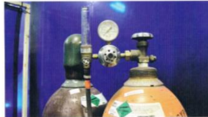
Exercise great caution when attaching a regulator to a cylinder.
