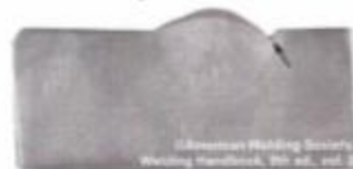
Undercut at the toe of an oxy-fuel arc weld
