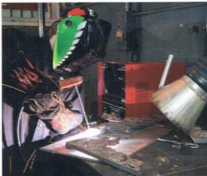
Welder using shielded metal arc welding
