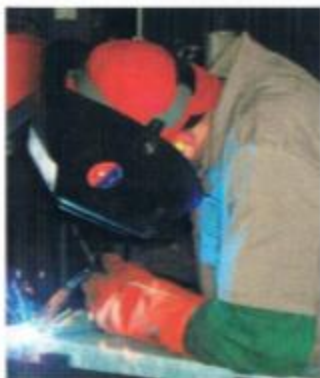
Gas metal arc fillet weld
