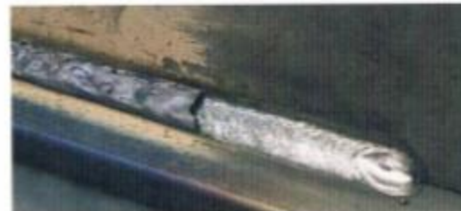
Slag peeling off shielded metal arc welding workpiece
