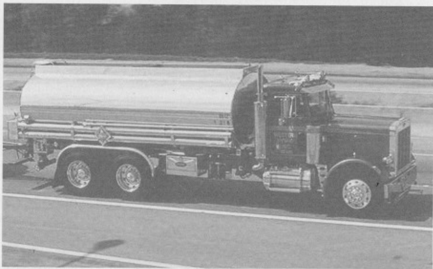
Tanker trucks are used to haul large amounts of liquid products, from milk and corn syrup to chemicals, gasoline, and heating oil.
