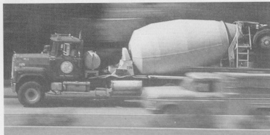
Cement mixers mix cement powder with water in a rotating barrel and haul the cement mixture to a construction site.
