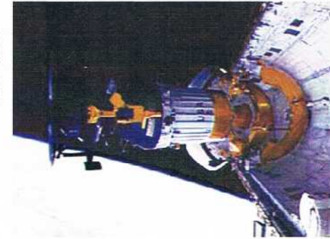
The Galileo spacecraft, carried aloft by the shuttle, weighed 2.5 tons. The shuttle can carry as much as 55,000 pounds of payload into an orbit about 100 miles high. The higher it goes, the less it can carry. At 320 miles above Earth, the shuttle's payload capacity drops to about 20,000 pounds.
