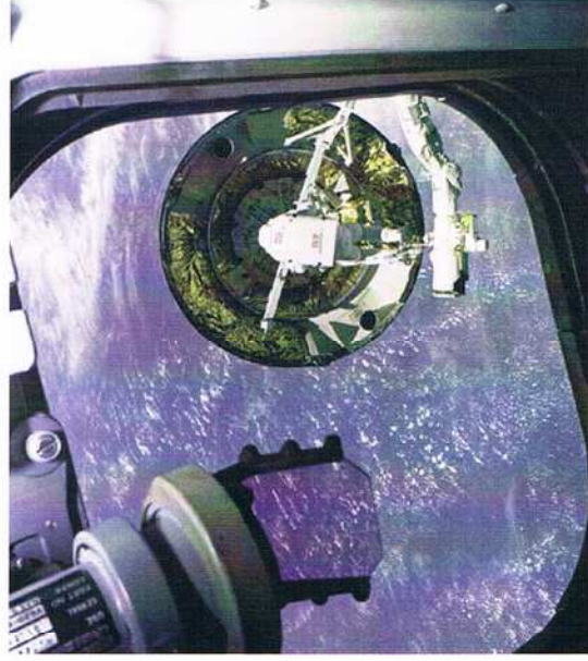
This photo, taken from the shuttle's aft (rear) flight deck windows, shows an astronaut from the space shuttle Endeavour trying to capture the Intelsat VI communications satellite.
