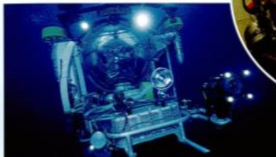
Submersibles are small, very deep-diving submarines that scientists use to explore ocean depths beyond the capabilities of scuba diving. Submersibles require a human pilot to guide them safely underwater.
