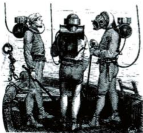
In 1860, Benoit Rouquayrol and Auguste Denayrouze introduced self-contained diving equipment that was essentially the same as that developed by Jacques-Yves Cousteau in the mid-20th century.
