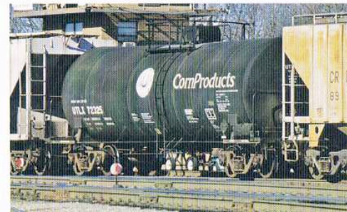
Tank cars carry liquids, mostly petroleum products such as fuel oil and petrochemicals, and liquids like vegetable oil, and are sometimes pressurized. Some tank cars have special linings to contain hazardous chemicals.
