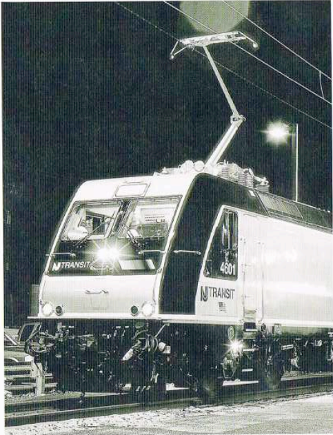
Electric locomotives (without a diesel engine) collect current from overhead wires, or catenary , through metal arms called pantographs mounted on the roof. Others use a pick-up shoe to collect current from an electrified third rail placed next to the running rails. The locomotive's internal equipment converts high-voltage current to lower voltage current.
