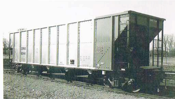
Open-top hoppers are used for freight like coal, mineral ores, sand, gravel, and crushed stone for track ballast.
