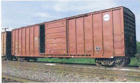
Enclosed railcars called boxcars range from 50 to 90 feet long and carry general freight in plain cars or products requiring special equipment or handling.
