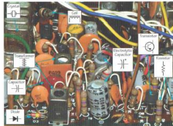
Electronic components with the schematic symbols that represent various parts
