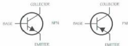
Schematic symbols for NPN and PNP transistors (Notice the arrow points in a different direction on each.)
