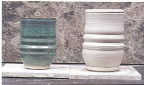
The fired piece at left shows the effects of shrinkage when compared with an identical piece, right, which has not yet been fired.
