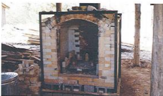
A typical fuel-burning kiln will take 12 to 24 hours to reach high-fire temperatures and another 24 hours to cool.
