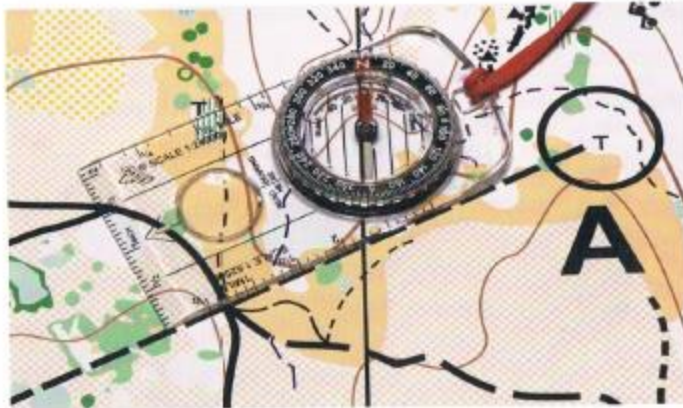
On the Sid Richardson Scout Ranch map, the compass edge is laid alongside the line from the hunter's stand at "A" and the northwest end of the cliff at "B." The bezel is turned until the north-south lines within the ring line up with the north arrow of the compass. Read the bearing from the index. The bearing is 244 degrees from "A" to "B." (Points "A" and "B" can be seen in the top photo on page 21.)
