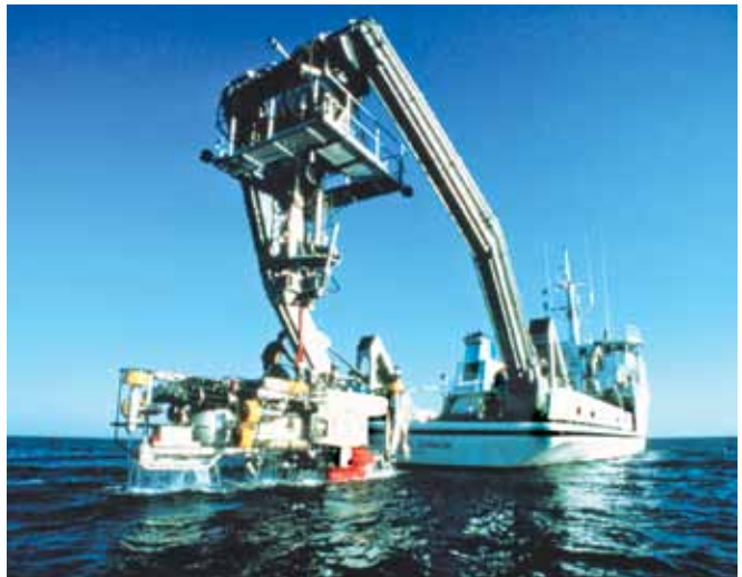
The Seward Johnson I , a research vessel, is prepared to deploy the submersible Johnson Sea-Link .
