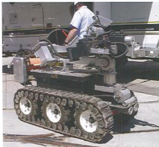
Mine rescue work uses a track-mounted robot to explore mines, reducing the need to send workers into potentially dangerous conditions.
