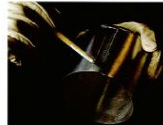
When using an acid flux, wear gloves and goggles, and work in an area with good ventilation.
