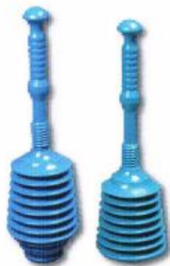
The bellows-style plunger for a toilet (left) has a narrowing plunging end to fit inside the bowl and create a better seal; those designed for flat drains (right) have a flat bottom to better seal a drain in a sink, tub, or basin.
