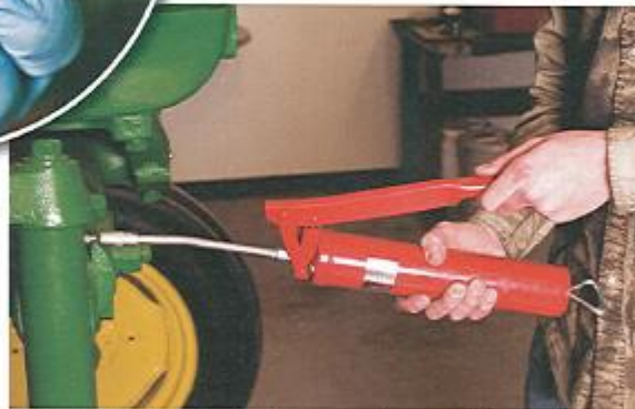
Follow the instructions in the operator's manual for greasing a machine. The manual will tell you how often grease is needed, where to put it, and what kind to use.
