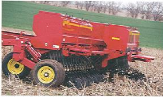
A grain drill plants small grains.
