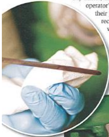
Transmission fluid level is checked with a dipstick. The operator's manual will specify the correct fill level and what type and weight of transmission fluid to use.
