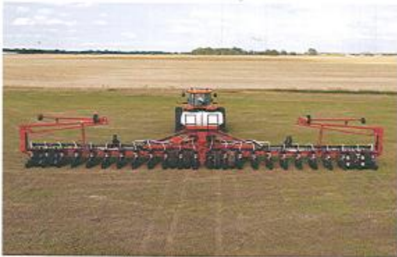
A grain drill plants small grains.
