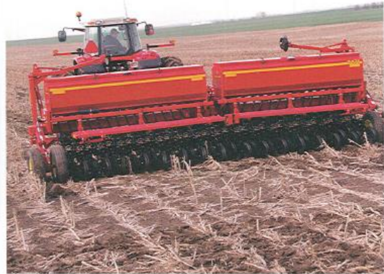
An air seeder combines tilling, seeding, and fertilizing in one field pass.
