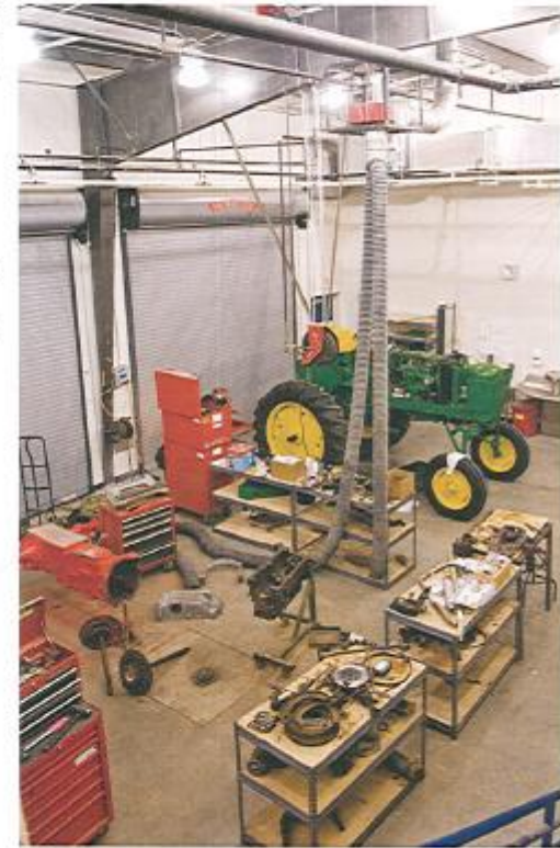
Workbenches, stationary tools, and main work areas should be well-lit.
