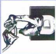
Poor connections look crystalline and grainy, or the solder tends to blob.
