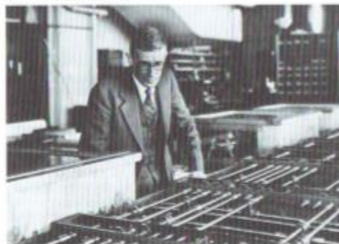
Massachusetts Institute of Technology engineer Vannevar Bush invented the differential analyzer, an electromechanical analog computer, in 1927.
