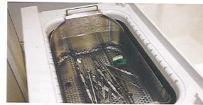
This ultrasonic cleaner sterilizes dental instruments.
