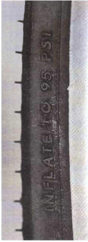
Tires should be kept inflated to the maximum pressure recommended by the manufacturer. This pressure is stamped on the side of the tire.
