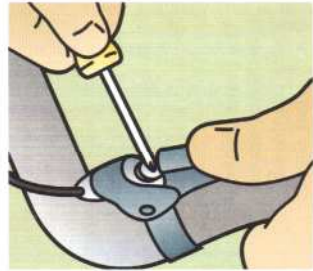
Squeeze the brake lever. Unscrew the barrel adjuster. This frees the cable for loosening or tightening. Increase or decrease cable tension using pliers. Holding the cable in place, screw in the barrel adjuster.
