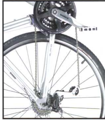
A good time to inspect the drive train and the rest of the bike for worn or broken parts is right after it has been cleaned.
