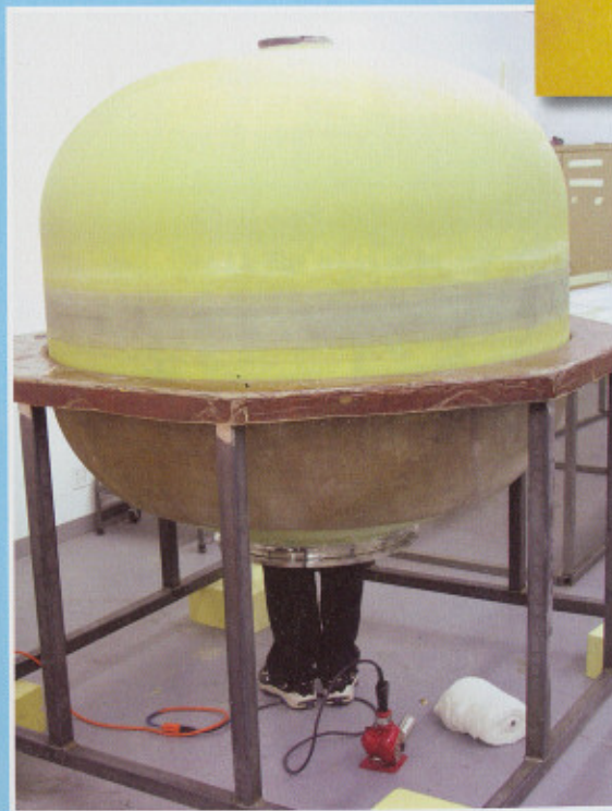
This worker completes additional graphite/epoxy lay-ups inside the nitrous tank used in SpaceShipOne.
