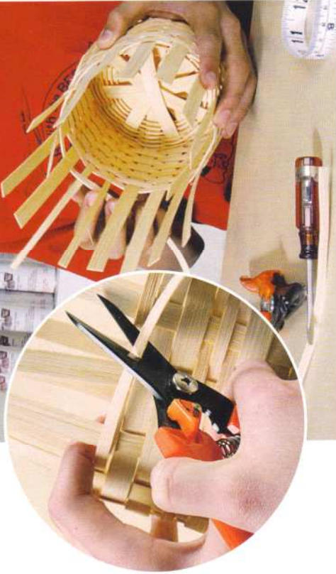
Point scissors and pliers away from your body when working with reed. Keep your bracing hand away from the path of the scissors.
