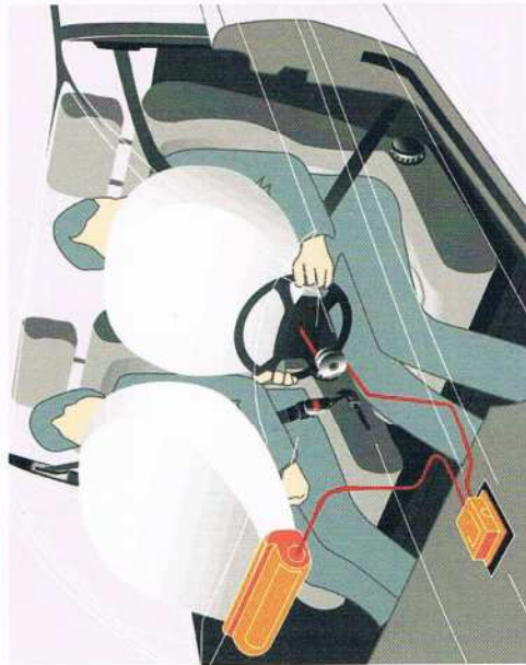
Air bags deploy automatically when a frontal crash occurs.
