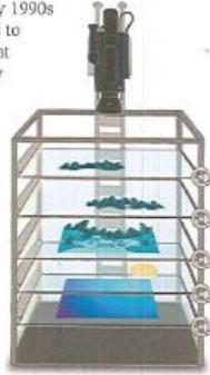
This illustration shows how the multiplane camera captures multiple "levels" of an image.
