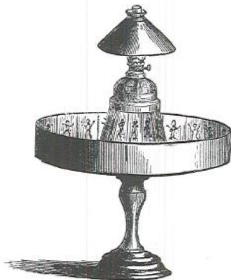
The praxinoscope improved upon the zoetrope by adding mirrors. Now the viewer didn't have to look through slits.
