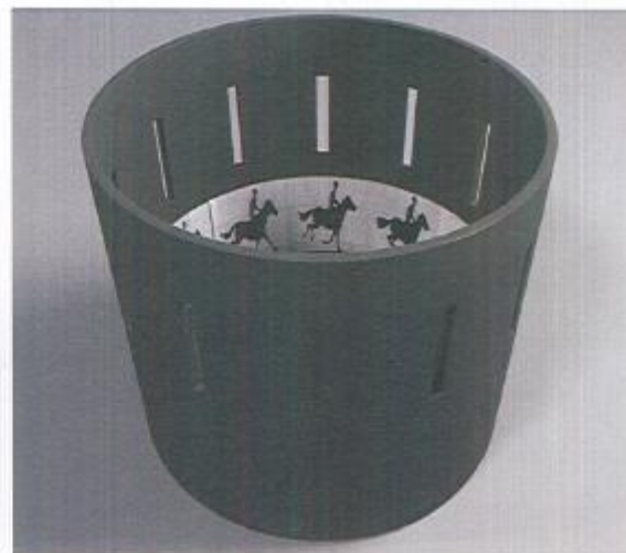
The zoetrope also relied on persistence of vision. If you look at the images through the slits while the drum is rotating, you see what appears to be a galloping horse.
